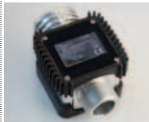
Type of output signal: raw signal (reed switch), single channel. Max 28 V Ac/dc 100 mAmp.
