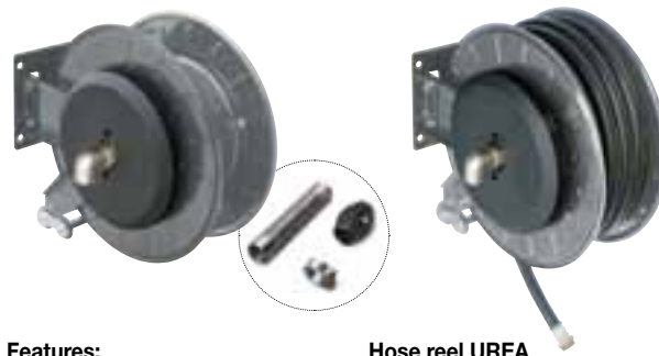
Features: - reduced pressure loss; - latch mechanism protective; - adjustable arms; - inlet with swivel 3/4" BSP - outlet hosedtail 3/4" BSP - Hose O 3/4" - Max hose length 8 m.
